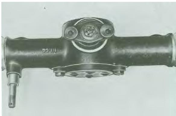
1. Remove hex retaining bolts from base plate and withdraw plate.
