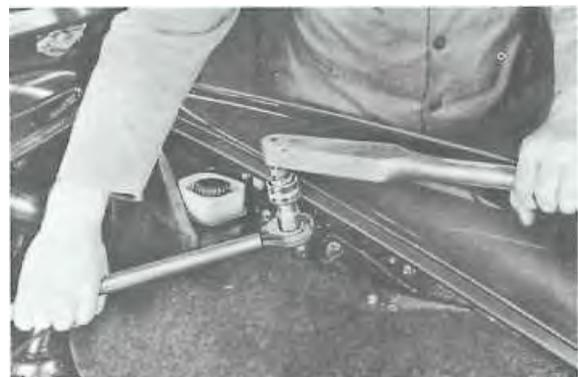
3. Remove ball joint retaining bolt (M 10 x 30) from strut and pull ball joint out of the strut by pushing the suspension control arm downward.
