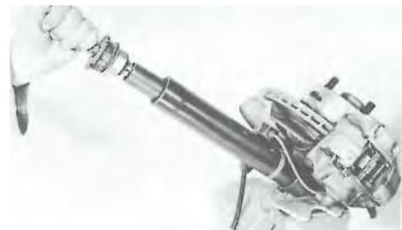
6. Drain the hydraulic fluid from the strut casing and install the new insert.
